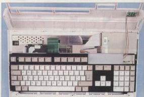
Step two: carefully release the ribbon connector and remove the keyboard
